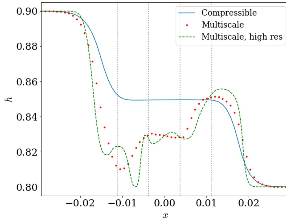
Multiscale dam break w/ 3 levels of (fixed) mesh refinement:
