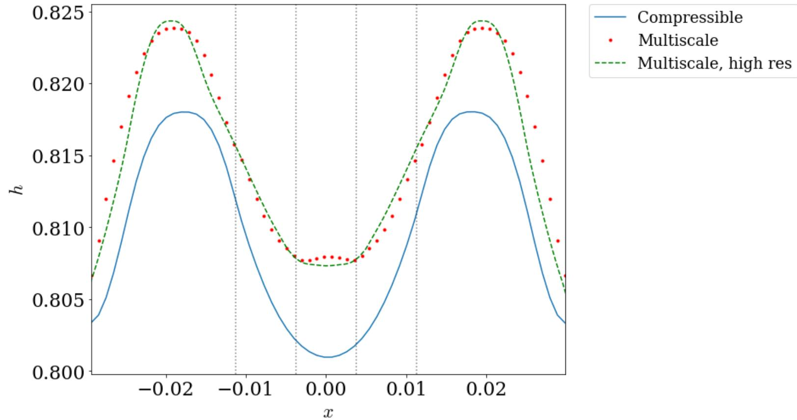
Multiscale Gaussian w/ 3 levels of (fixed) mesh refinement: 1 coarse SW level, 2 finer compressible levels centred about  $x = 0$  (see dotted grey lines)
